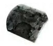
Dirt on the brake lining surface
