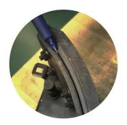
Build up dirt between lining and brake shoe
